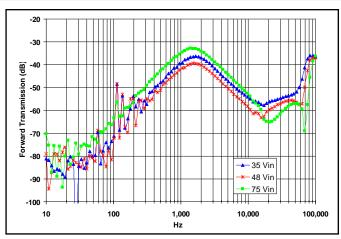
Figure 18: Magnitude of incremental forward transmission (FT = v<sub>out</sub> vin) for minimum, nominal, and maximum input voltage at full rated power.
