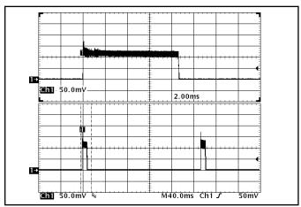
Figure 15: Load current (5A/div) as a function of time when the converter attempts to turn on into a 10 m $\Omega$  short circuit. Top trace (2ms/ div) is an expansion of the on-time portion of the bottom trace.
