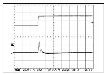
Figure 16: Output voltage response to step-change in input voltage (1000V/ms). Ch1: Vin (20V/div), Ch2: Vout (1V/div).
