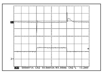
Figure 9: Output voltage response to step-change in load current (50%-75%-50% of Iout(max);  $dI/dt = 0.1A/\mu s$ ). Load cap:  $15\mu F$ , 450 m $\Omega$  ESR tantalum cap and 1µF ceramic cap. Top trace: Vout (500mV/div), Bottom trace: Iout (5A/div).
