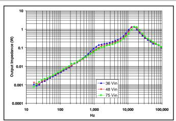
Figure 17: Magnitude of incremental output impedance ( $Z_{out} = v_{out}$ ) i<sub>out</sub>) for minimum, nominal, and maximum input voltage at full rated power.
