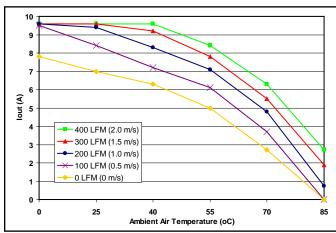
Figure 5: Maximum output power derating curves (no heatsink) vs. ambient air temperature for airflow rates of 0 LFM through 400 LFM with air flowing from pin 3 to pin 1 (nominal input voltage).
