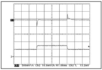
Figure 10: Output voltage response to step-change in load current (50%-75%-50% of Iout(max):  $dI/dt = 5A/\mu s$ ). Load cap:  $480\mu F$ , 15 m $\Omega$  ESR tantalum cap and 1µF ceramic cap. Top trace: Vout (500mV/div), Bottom trace: Iout (5A/div).
