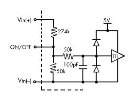
Figure B: Internal ON/OFF pin circuitry
