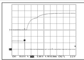
Figure 7: Turn-on transient at full load (resistive load) (10 ms/div). Input voltage pre-applied. Top Trace: Vout (10V/div). Bottom Trace: ON/OFF input (5V/div).
