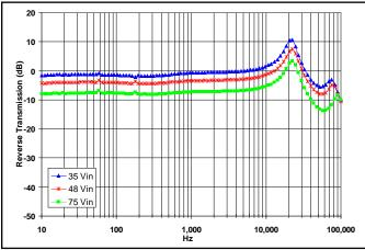
Figure 19: Magnitude of incremental reverse transmission (RT =  $i_{int}/i_{out}$ ) for minimum, nominal, and maximum input voltage at full rated power.
