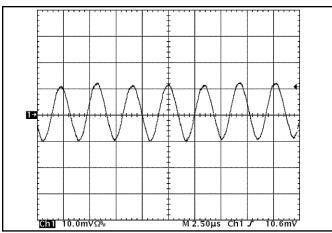
Figure 13: Input reflected ripple current,  $i_s$ , through a 10  $\mu H$  source inductor at nominal input voltage and rated load current (10 mA/div). See Figure 11.
