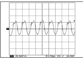
Figure 14: Output voltage ripple at nominal input voltage and rated load current (20 mV/div). Load capacitance: 1µF ceramic capacitor and 15µF tantalum capacitor. Bandwidth: 20 MHz. See Figure 11.
