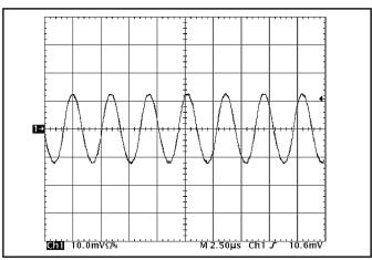
Figure 12: Input Terminal Ripple Current, ic, at full rated output current and nominal input voltage with  $10\mu H$  source impedance and  $47\mu F$ electrolytic capacitor (500 mA/div). See Figure 11.
