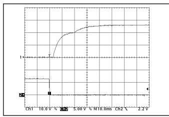
Figure 8: Turn-on transient at zero load (10 ms/div). Top Trace: Vout (10V/div). Bottom Trace: ON/OFF input (5V/div).
